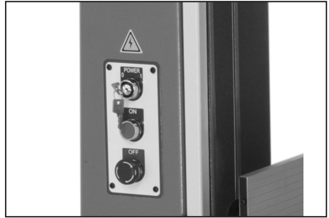
Figure 20. G0636X switch disabling key and ON/OFF switch.
